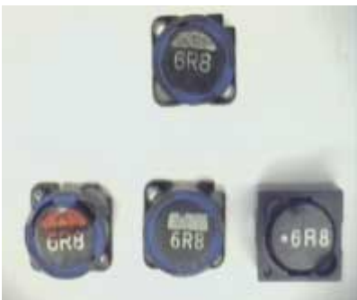
The first (oldest version with soldering problem)
